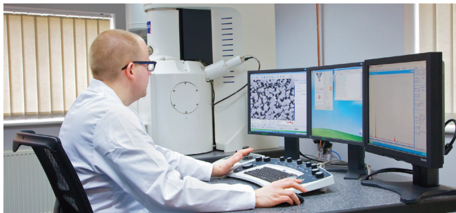
Figure 1. Advanced microscopy enables the surface characteristics of the substrate to be examined and photographed for comparison to that of treated samples.
