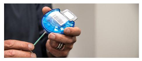
Professor Chris Toumazou FREng FRS FMedSci of Imperial College London for developing a rapid, affordable COVID-19 test based on a lab in a cartridge technology that provides test results in just over an hour. A total of 5.8 million tests are now being deployed throughout NHS in preparation for the flu season. ©thisisjude.uk 2020
