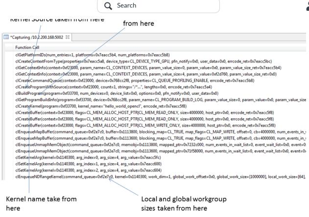
obtain the information from clCreateKernelsInProgram. As shown in the image above MGD also captures the build options used in clBuildProgram to pass to GPUVerify. The more details that can be passed to GPUVerify the more accurate it can analyze your kernels.
