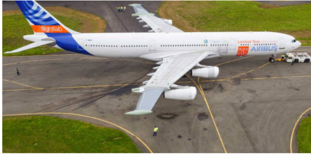
BLADE wing extensions on this A340 aid laminar flow research at Airbus.
