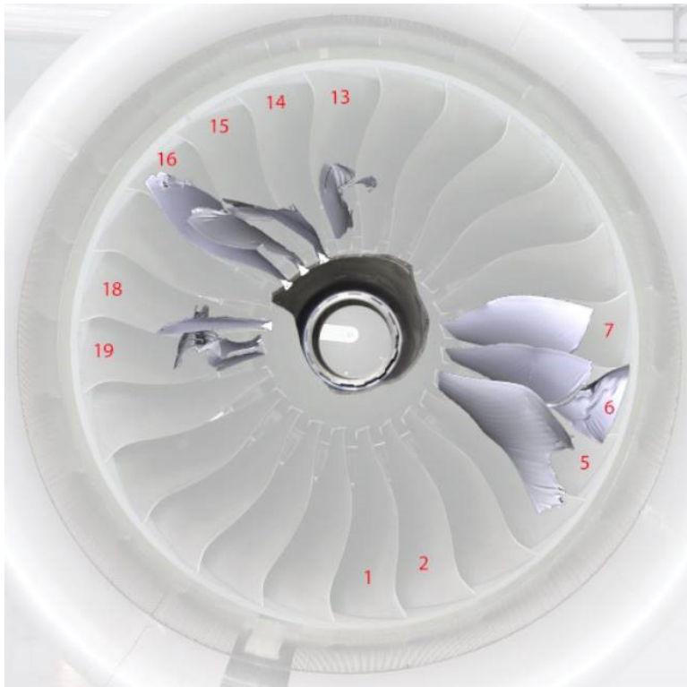
Figure 7: Illustration of fan blades found, when their position is known. Blades 5, 6, 7, 13, 14, 15, 16 and 19 were found on the Greenland ice sheet. Blade 18 was found embedded in the OGVs. The fragments found in the engine at Goose Bay no longer had any identification numbers and could not be positioned on the engine. Position 1 was chosen arbitrarily at the bottom of the engine for illustration purposes.
