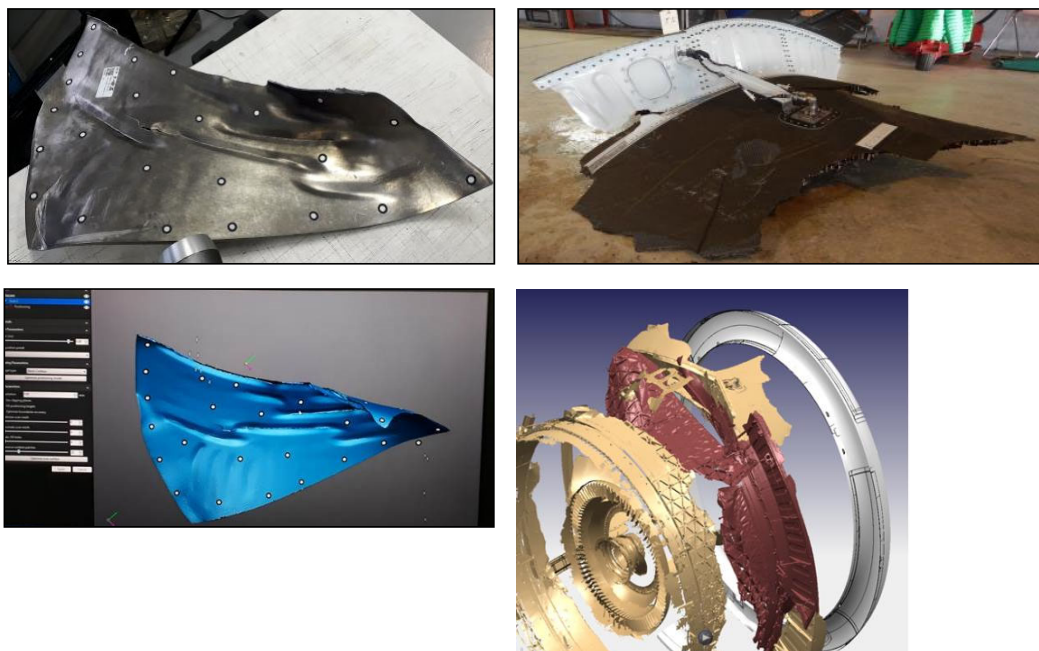
Figure 14: fan blade during scan (top left) and result of scan (bottom left). Part of inlet cowl aft bulkhead (top right) and result of scan (in red, bottom right) inserted in a more complete 3D model of the damaged engine.
