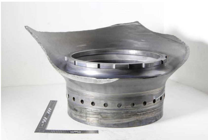
Figure 11: Hub fragment after its removal from damaged engine
