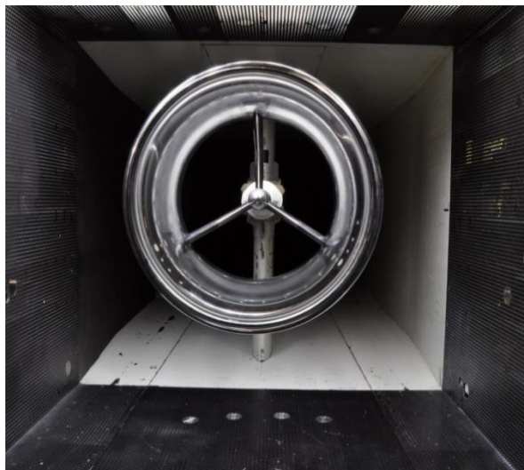
Figure 1: Ring wing model installed in the ARA TWT
