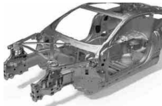
Impression Technologies has a vital role in the Aston Martin DB11's new aluminium bonded structure.
