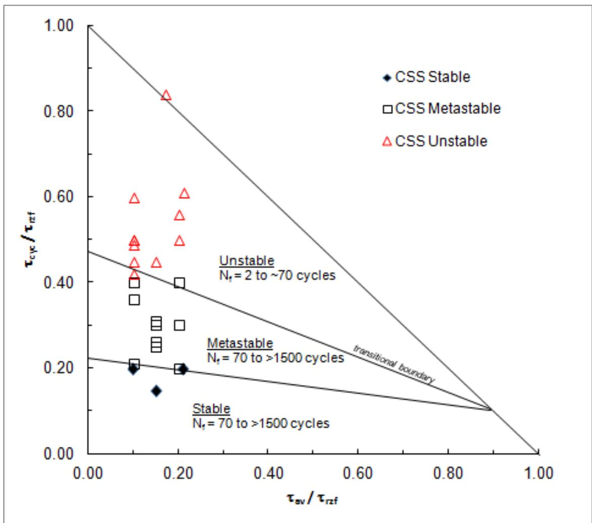
**Figure 3-2:** Illustration of potential cyclic stability zones in a normalised cyclic interaction diagram
