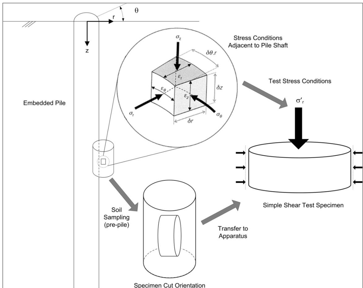
**Figure 3-1:** Schematic of stress conditions in a soil element adjacent to a pile shaft as translated in the direct simple shear test (see also Sim et al., 2013)
