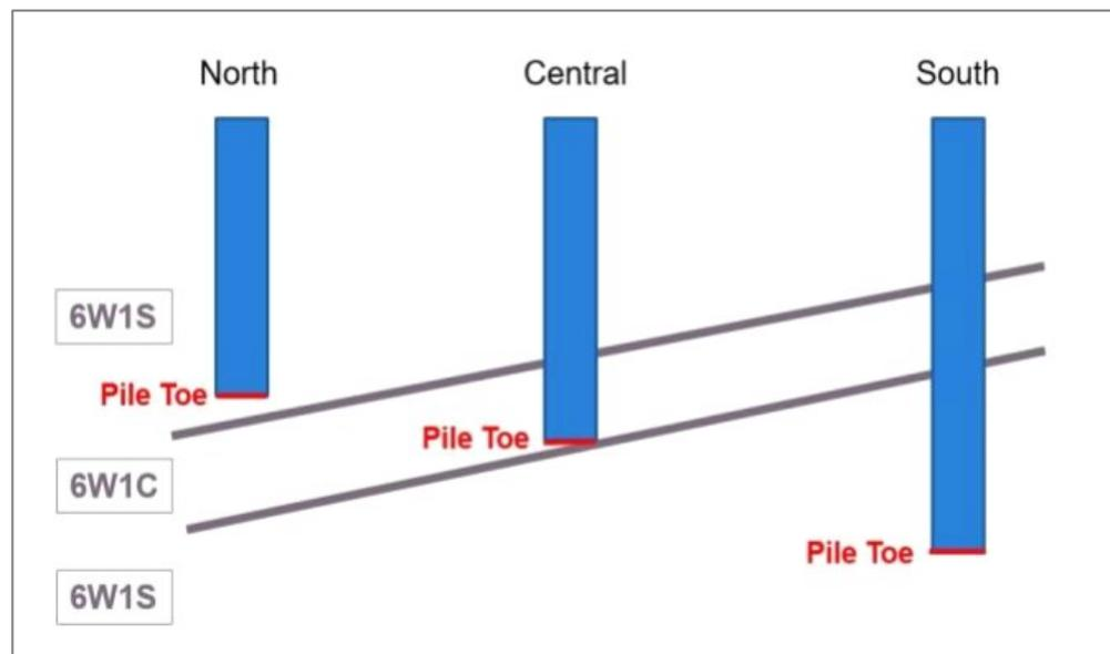
**Figure 2-1:** Illustration of pile tipping layer across EAONE
